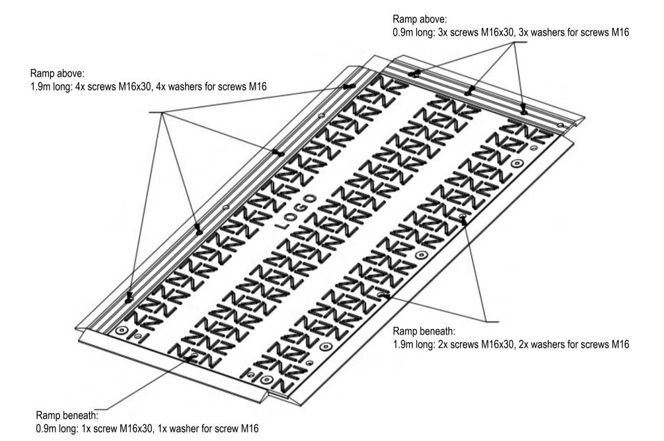
The design of the ramps installed above or beneath the panels, regardless of whether they are used for the vehicle or pedestrian side, is identical. Only the number of connection options differs on the vehicle and pedestrian sides.
