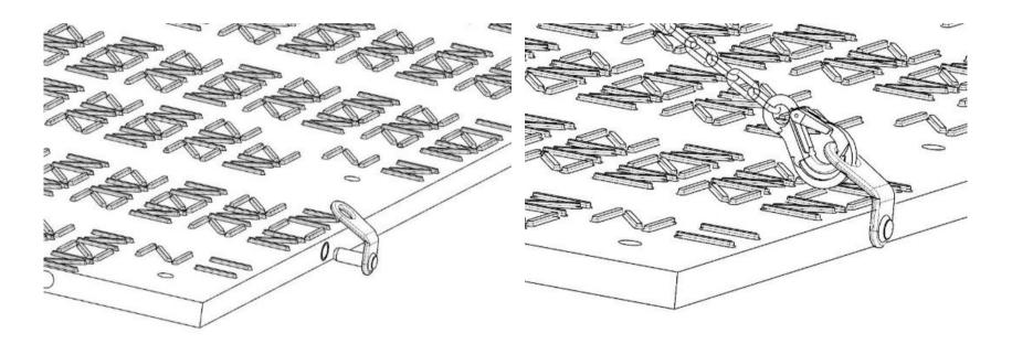
With the help of the chain sling, the panel can be moved to the desired position and installed.
