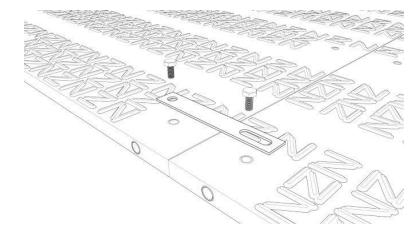
Care should be taken when laying the panels to ensure that they have the same profile side facing up.
