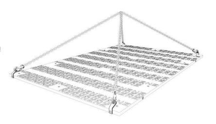
Insert the load-bearing hooks in the lifting lugs on the side to be able to move the panel optimally using a chain sling and to bring it into the desired position.
