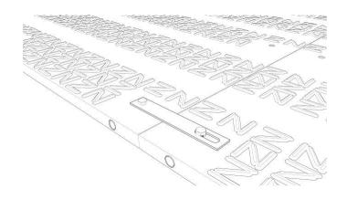
Lay the panels next to each other and bolt them to create a construction road or work platform with the desired traction capacity.
