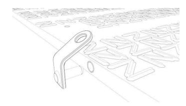
The panel is transported or laid in the desired position by tightening the chain sling so that it can then be bolted.
