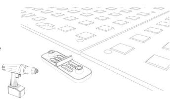
Joining the panels together produces a contiguous surface that protects the ground and distributes pressure when driving on the surface with vehicles.
