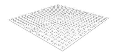
To screw the panels together, simply insert the connectors underneath the panels and then secure them with an M10x25 screw and washer from above.
