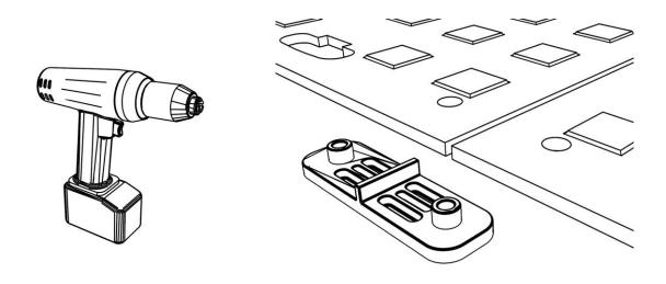
Joining the panels together produces a contiguous surface that protects the ground and distributes pressure when driving on the surface with vehicles.
