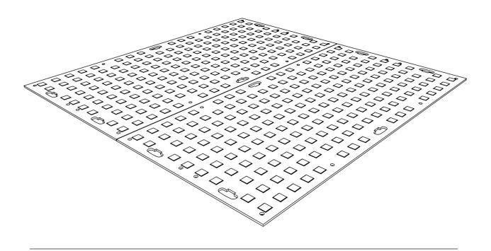
To screw the panels together, simply insert the connectors underneath the panels and then secure them with an M10x25 screw and washer from above.
