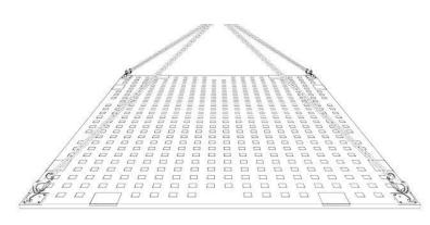
Insert the load-bearing hooks in the lifting lugs on the side to be able to move the panel optimally using a chain sling and to bring it into the desired position.
