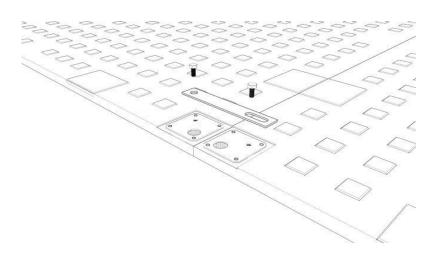
Care should be taken when laying the panels to ensure that they have the same profile side facing up.
